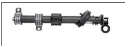
Figure 9.7 Bayonet type assembly
